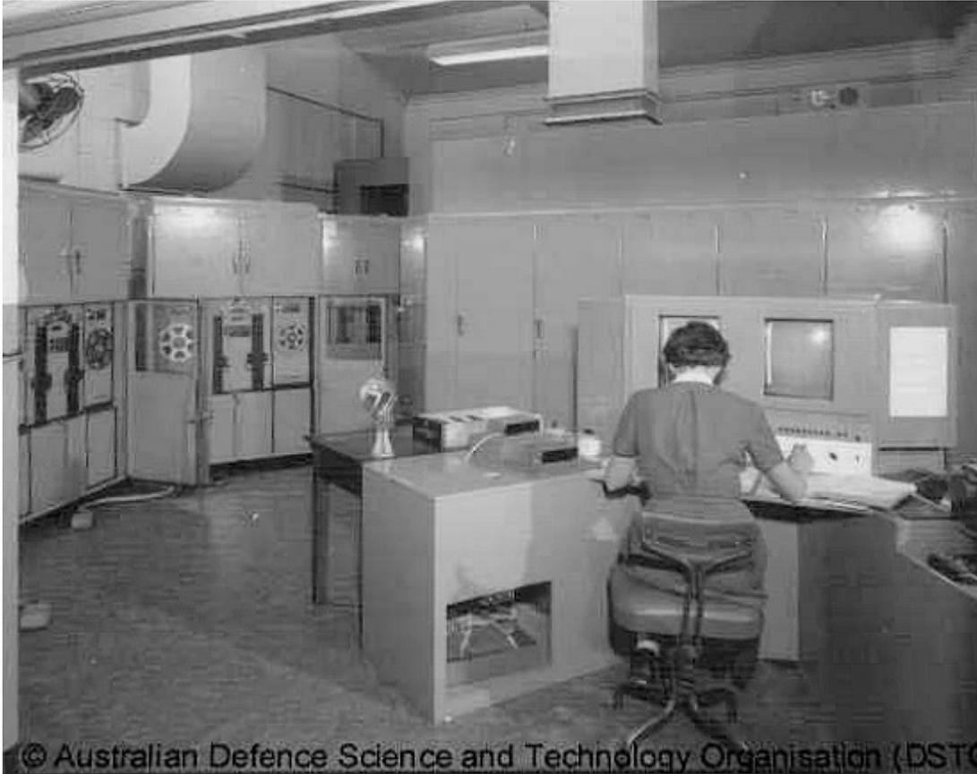
WREDAC, showing the replacement console designed and built by WRE engineers.
